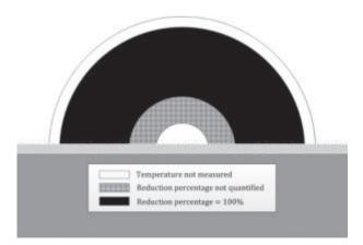
**Figure 7.4.** Estimated temperature profiles inside the dunghill at Farm A on 4th November 2009. Cases for  $Q_{prod} = 0$  (only conduction, equation 3) and for  $Q_{prod} = 50$  W/m<sup>3</sup> and  $\lambda = 2$  W/m·K (conduction and heat production, equation 2) are shown. The  $\lambda$  value of wet soil is taken (Mills, 1999), the value for  $Q_{prod}$  was estimated based on heat transfer calculations using the outdoor air temperature on 4<sup>th</sup> November 2009.
