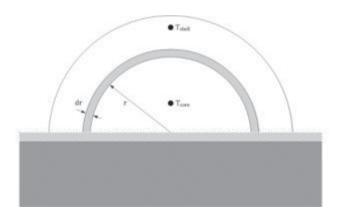
**Figure 7.1a.** Schematic drawing of dunghill cross section, placed on a concrete floor. Please note that in reality the shape of a dunghill is less smooth. Calculations were performed with a height of the dunghill of 2.5 m, a width of 5 m, and a length (into the paper) of 10 m. These dimensions approach those of the dunghill of farm A. The measurement locations for shell and core temperatures are indicated. r = radius [m], T = temperature [°C].
