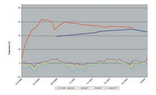
**Figure 7.3b.** Temperatures in the core (dark blue) and shell (red) of the dunghill on farm B. The average (yellow), the minimum (turquoise) and the maximum (purple) outside temperature in Eindhoven, the Netherlands (www.knmi.nl) during the experiments are shown. All temperatures are in degree Celsius.
