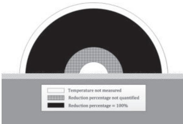
**Figure 7.4.** Estimated temperature profiles inside the dunghill at Farm A on 4th November 2009. Cases for  $Q_{prod} = 0$  (only conduction, equation 3) and for  $Q_{prod} = 50 \text{ W/m}^3$  and  $\lambda = 2 \text{ W/m-K}$  (conduction and heat production, equation 2) are shown. The  $\lambda$  value of wet soil is taken (Mills, 1999), the value for  $Q_{prod}$  was estimated based on heat transfer calculations using the outdoor air temperature on 4<sup>th</sup> November 2009.
