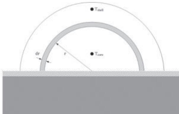
**Figure 7.1a.** Schematic drawing of dunghill cross section, placed on a concrete floor. Please note that in reality the shape of a dunghill is less smooth. Calculations were performed with a height of the dunghill of 2.5 m, a width of 5 m, and a length (into the paper) of 10 m. These dimensions approach those of the dunghill of farm A. The measurement locations for shell and core temperatures are indicated.  $r$  = radius [m],  $T$  = temperature [ $^{\circ}\text{C}$ ].
