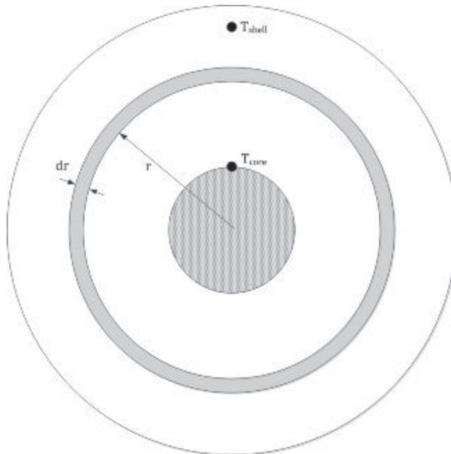
**Figure 7.1b.** Schematic drawing of dunghill as simplified for setting up an energy balance. The dunghill was modelled as a hollow cylinder of infinite length with an inner radius of 0.5 m and an outer radius of 2.5 m. Temperature prediction was only possible between both temperature measurement locations ( $T_{core}$  and  $T_{shell}$ ).  $r$  = radius [m],  $T$  = temperature [°C].
