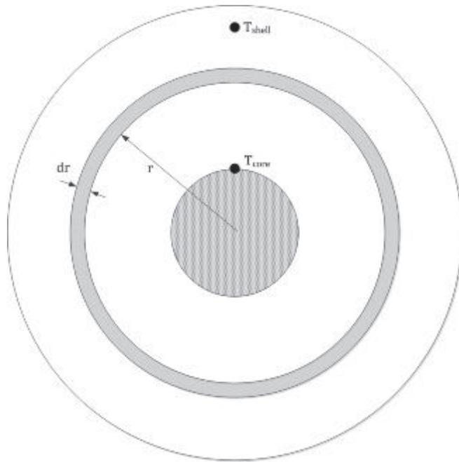
**Figure 7.1b.** Schematic drawing of dunghill as simplified for setting up an energy balance. The dunghill was modelled as a hollow cylinder of infinite length with an inner radius of 0.5 m and an outer radius of 2.5 m. Temperature prediction was only possible between both temperature measurement locations ( $T_{core}$  and  $T_{shell}$ ).  $r$  = radius [m],  $T$  = temperature [ $^{\circ}$ C].
